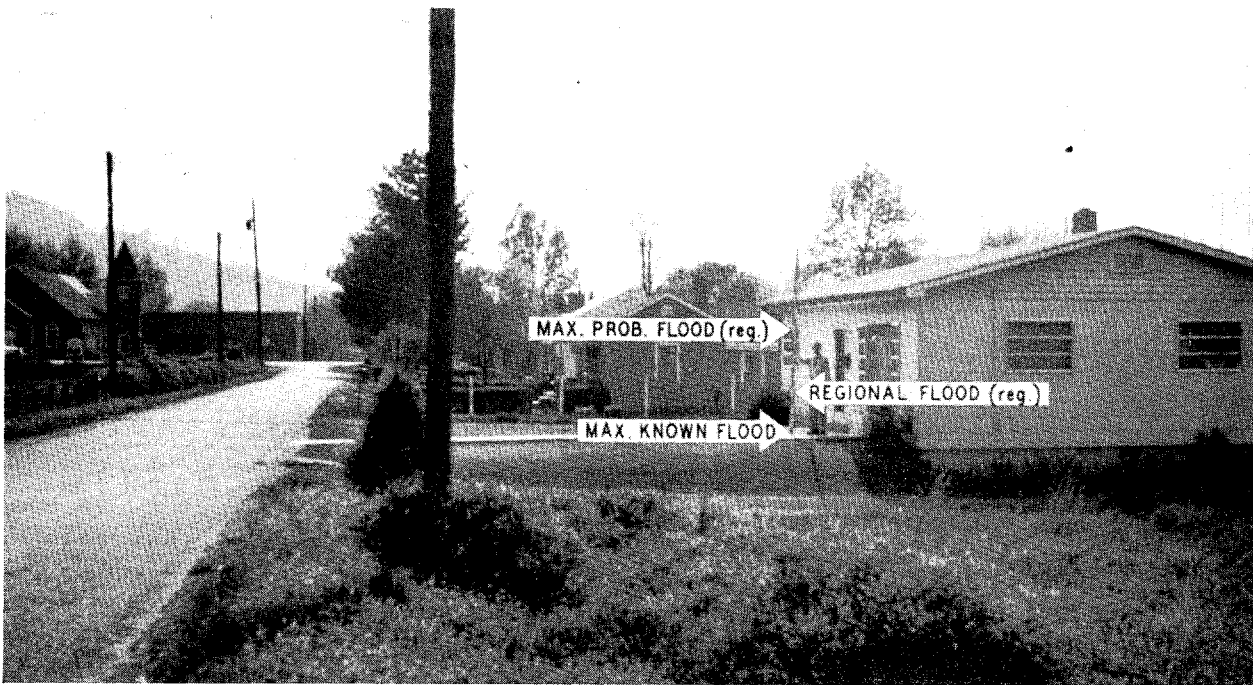
Figure 12. --FLOOD HEIGHTS ON NORTH AVENUE
